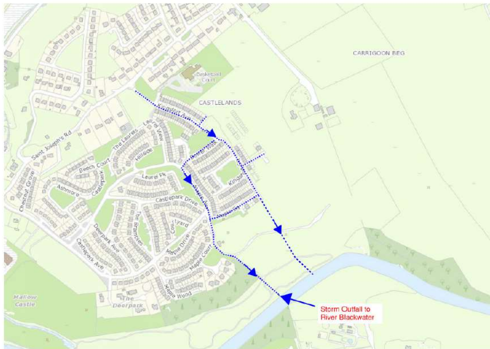
FIGURE 2. SHOWING THE LOCATION OF THE STORMWATER OUTFALL TO THE BLACKWATER RIVER FROM RESIDENTIAL ESTATE ADJACENT TO THE PROPOSED DEVELOPMENT (DOSA CONSULTING ENGINEERS, 2024).
