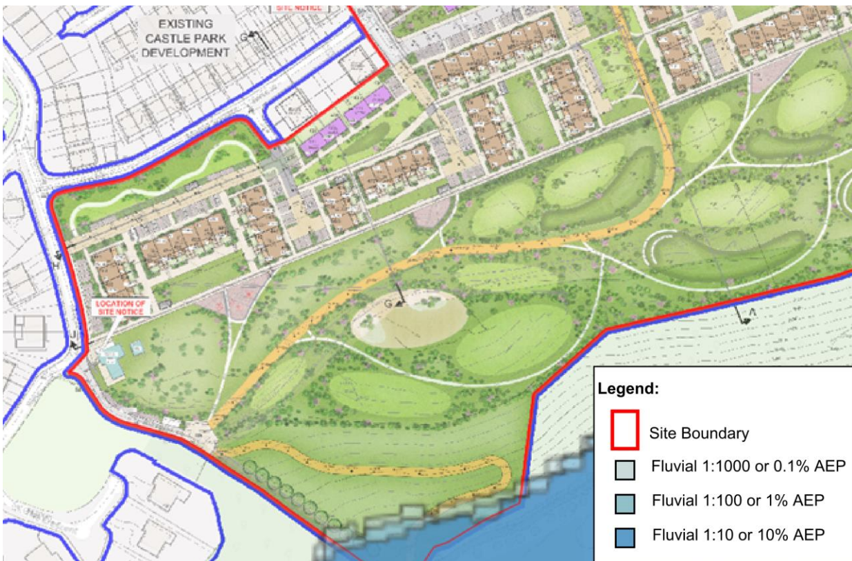
Figure 8 South Western CFRAM Study Fluvial Flood Extent Map, current, overlaid on architectural plans
