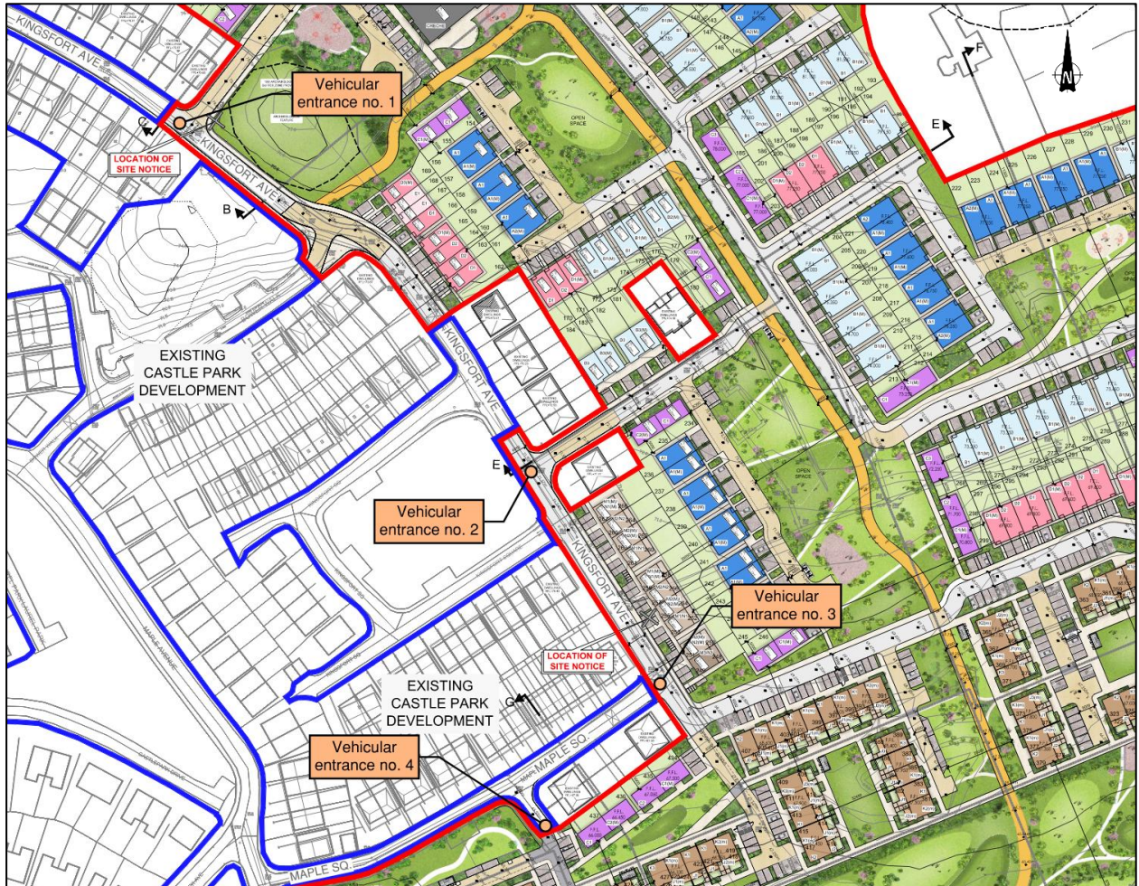
Figure 6-2 Site Layout Extract showing Access Arrangements
