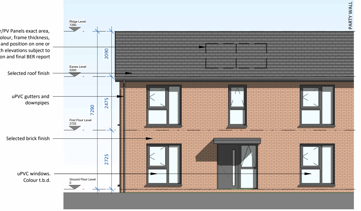
Front Elevation SCALE 1 : 100
