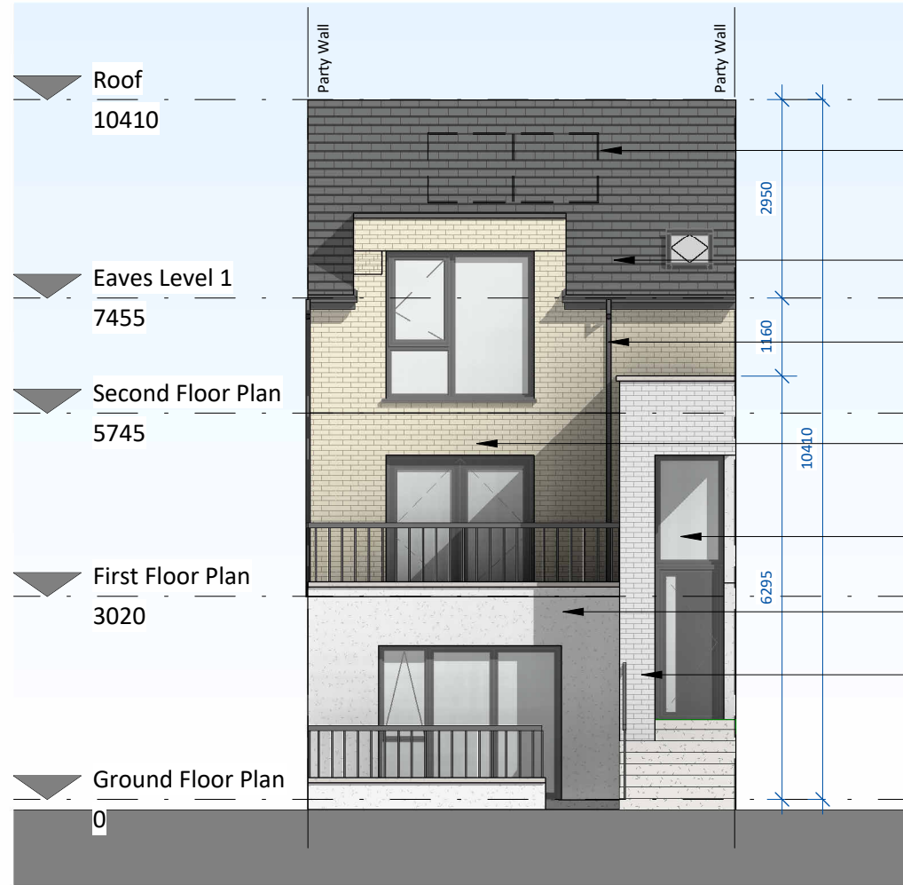
Front Elevation. SCALE 1 : 100
